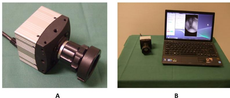
**Figure 1.** Fastec HiSpec1 without (A) and with (B) laptop displaying a captured image.
